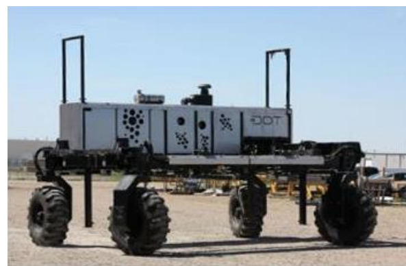
The DOT powered platform is an autonomous tool carrier. | Michael Raine photo
