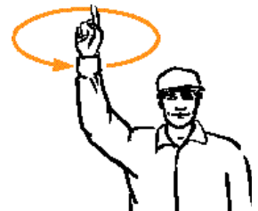
RAISE EQUIPMENT – Point upward with forefinger, making a circle at head level with your hand.
